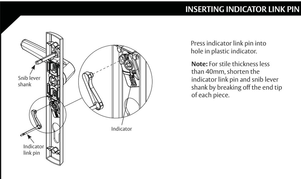
Press indicator link pin into hole in plastic indicator.
