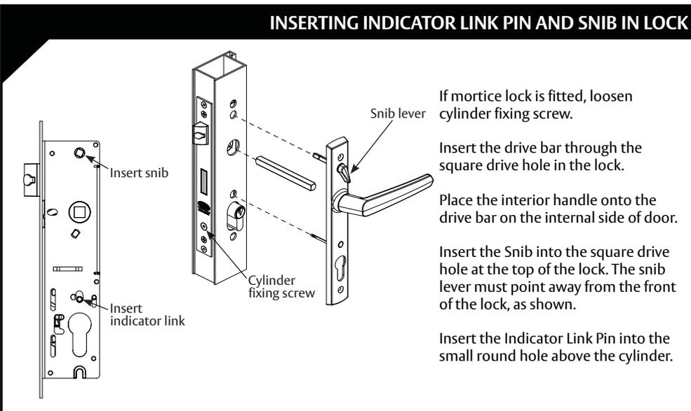
If mortice lock is fitted, loosen cylinder fixing screw.
