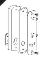
• Fit the rubber mounting pad onto the mounting plate and then secure to the DX digital unit using supplied 10mm long screws.
