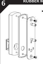
• Fit the rubber mounting pad onto the mounting plate and then secure to the DX digital unit using supplied 10mm long screws.
