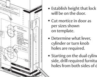
Starting on the dual cylinder side, drill required furniture holes from both sides of door.
